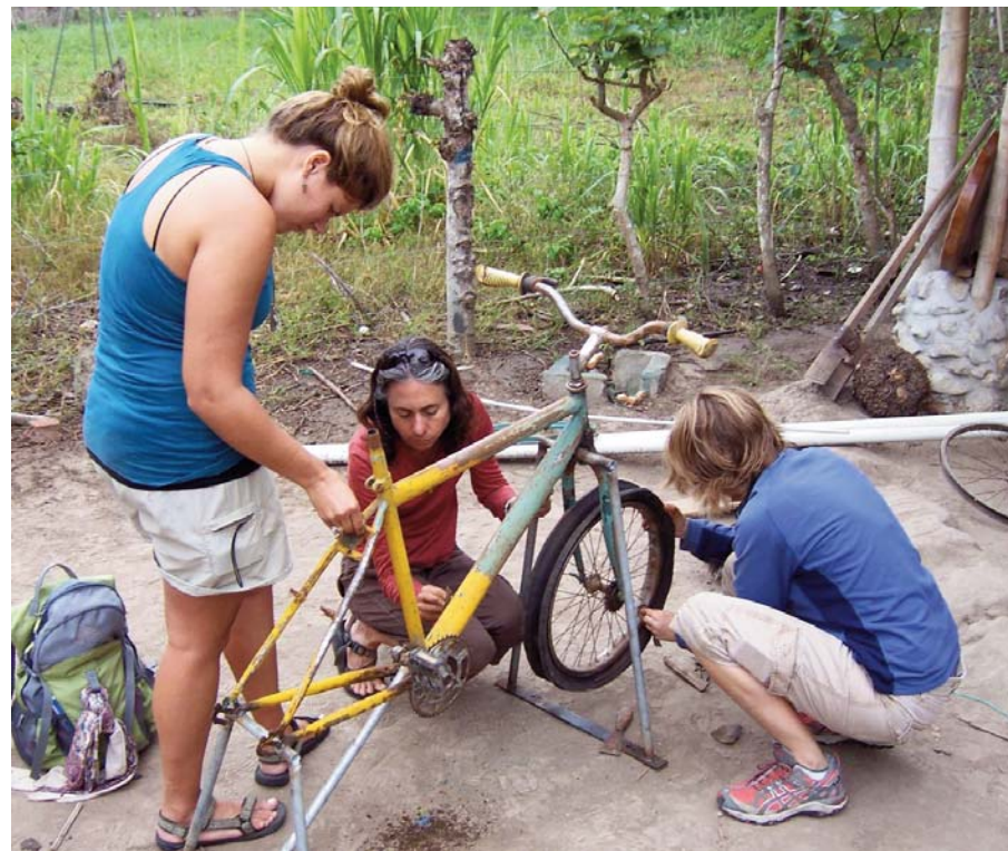
Building a bicycle powered water pump in the Ecology, Permaculture, & Renewable Energy workshop in Ecuador. ▼
