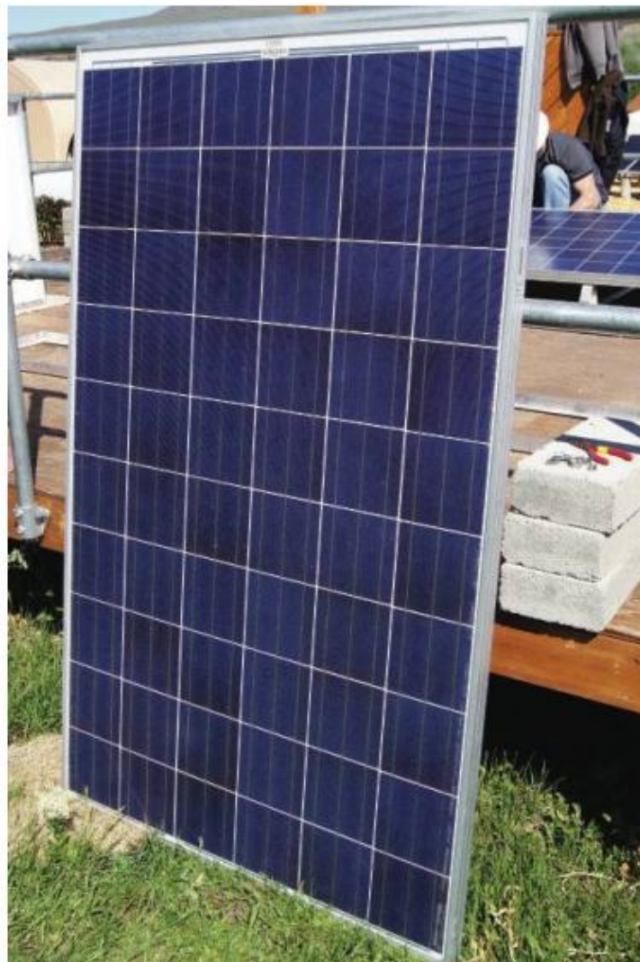
Figure 4.1: PV modules generate dc electricity from sunlight.
